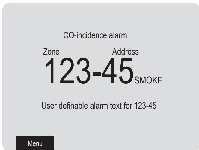
If more than one Co-incidence alarm not dependent on each other are activated, the LEDs "Alarms queued" are blinking and the Coincidence alarms will be automatically scrolled (every five seconds).
