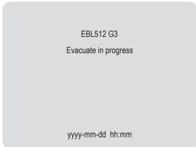
Alternatively, the same is the result when an input programmed as "Evacuate" is activated. One input per CIE.
