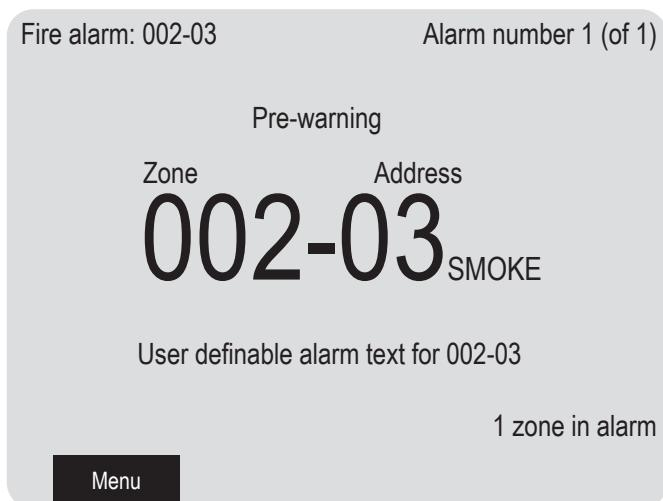
After the presentation number is automatically added SMOKE, HEAT, MULTI or MCP depending on type of alarm source, for more information see section [18.2. ALARM SOURCE](#) on page 49.
