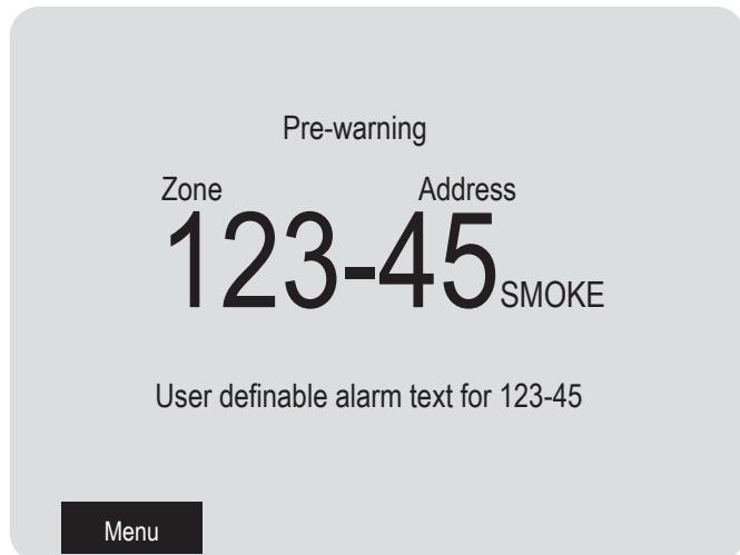
"SMOKE" after the presentation number is automatically added depending on the type of alarm point (SMOKE, HEAT, MULTI or MCP).
