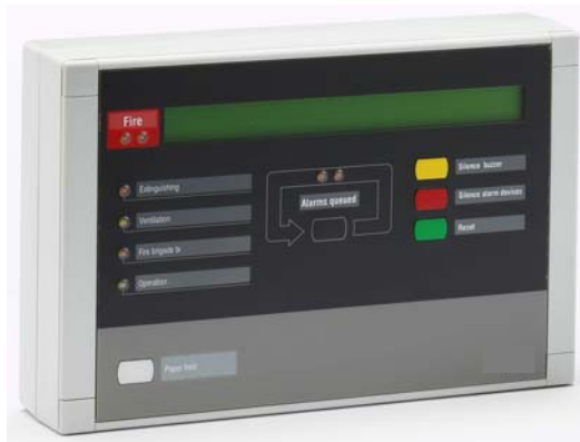
Figure 2. The Alert Annunciation unit 1736. A neutral front where the designation texts, by production, are made separately and put into the transparent "text slot" for the LED and push button respectively. (It also holds one extra LED & two extra push buttons.)
