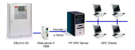
The FP OPC Server is a Panasonic software that runs on a PC or a server. The Web-server II 1598 (with software OPC512 G3) is a gateway between the fire alarm system and the FP OPC Server. The OPC clients are communicating with the FP OPC Server via an interface described in this document.
