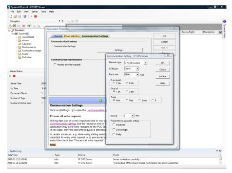
For serial settings one should set network type to 'C-NET (RS232)' and then select COM port, baud rate etcetera. Automatic settings are not supported so the three checkboxes in the bottom should be unchecked.
