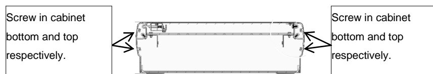
Figure 5. Four screws in the cabinet bottom and four screws in the cabinet top have to be unscrewed to get access to the rail fixing screws.
