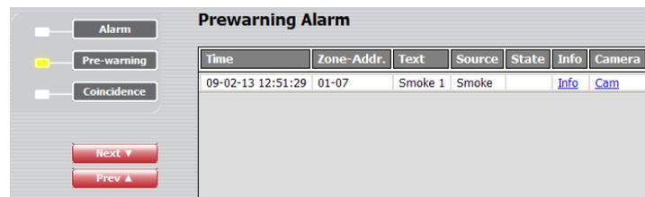
The **Time** (date & time), **Zone – Address** and **Text** (alarm text) are displayed.
