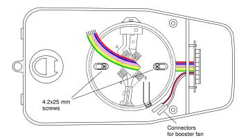
Connect Uniguard wires to the base
