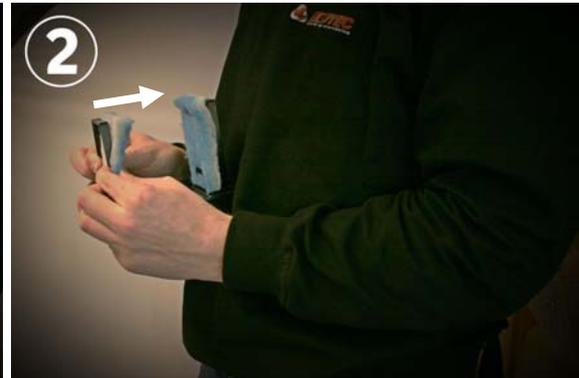
Finally, reinstall the cartridge, making sure that it is fitted tightly. Use your thumb to feel that the cartridge front is flush with the two raised areas of the filter housing.
