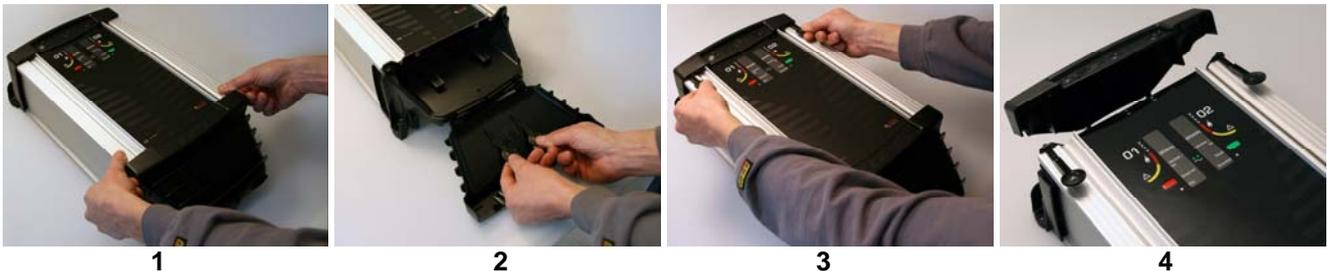
1. Open the bottom cover by grasping the recesses in its upper edge, pulling forward and down.
