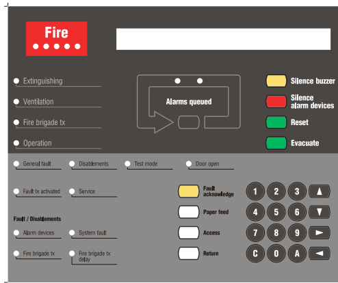
Figure 2. The EBL512 front; FBP (upper dark grey part) and CP (lower light grey part). The look might vary according to country, language, convention and configuration (e.g. English texts as in the figure).
