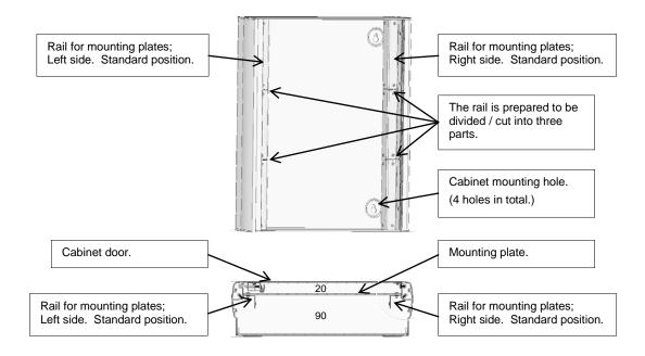
When the rails are mounted for standard position of the mounting plates (like in the figure), the free space behind the plate is approx. 90 mm and in front of the plate approx. 20 mm.
